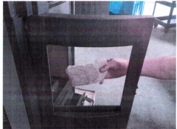
Figure 31: Wipe glass and inspect gasket
